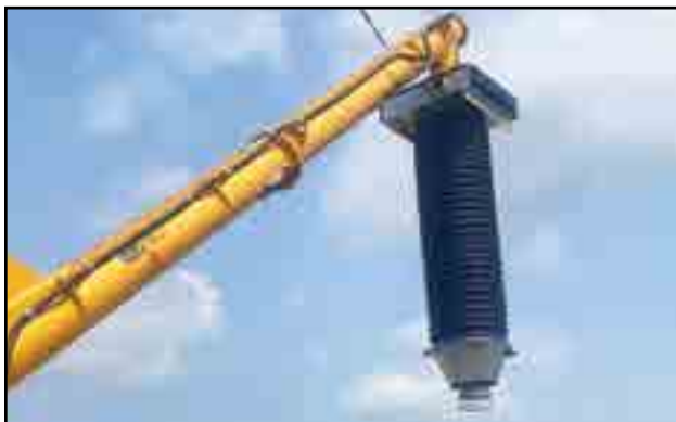
Fig 32 - Bellows/retractable downspout for auger
