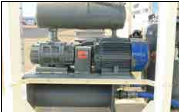
Fig 22 - 7.5 HP Air compressor
