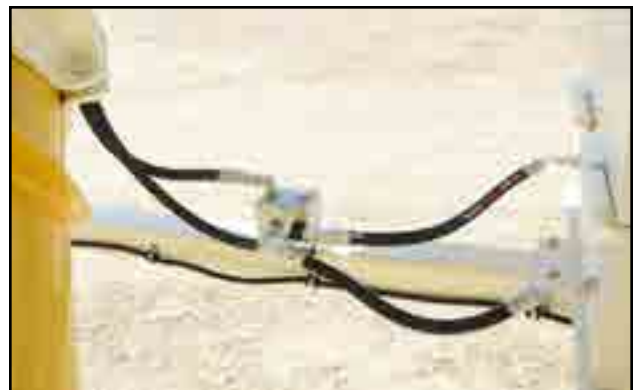
Fig 30 - Check valve to auger unfolding cylinder
