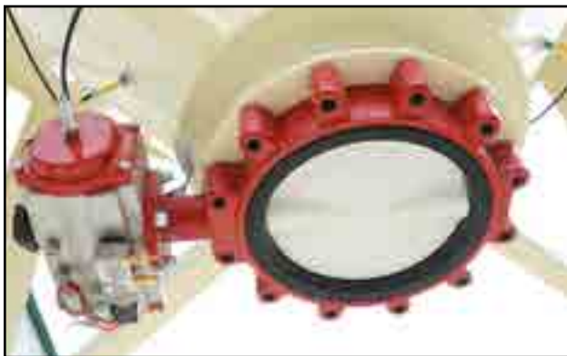
Fig 33 - 12" Butterfly valve without auger attached
